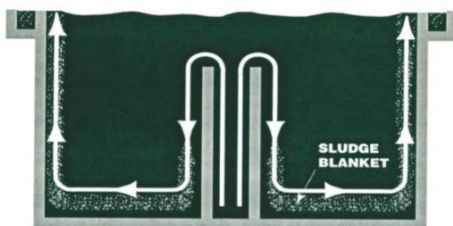
Figure 1. Density Currents in an Activated Sludge Clarifier
